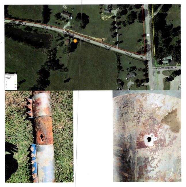
Dade County Water & Sewer Authority has purchased 200 LF of C-900 high pressure Polyvinyl Chloride pipe to replace the section that is directly across from the rectifier. C-900 pipe is not conductive and will prevent the stray direct current from eroding the remainder of the existing pipe.
